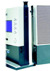
Figure 5-2: Attaching the Right Speaker
